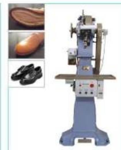
UN-S619 Double needle welt sewing machine
