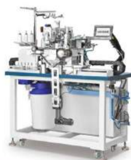
GK-375S Automatic underwear elastic waistband attaching machine
