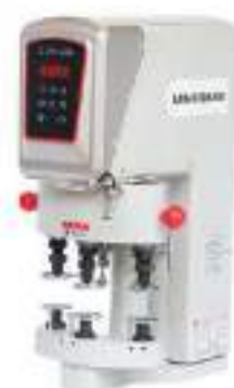
UN-T3 Direct drive snap button attaching machine UN-T3 electric type
