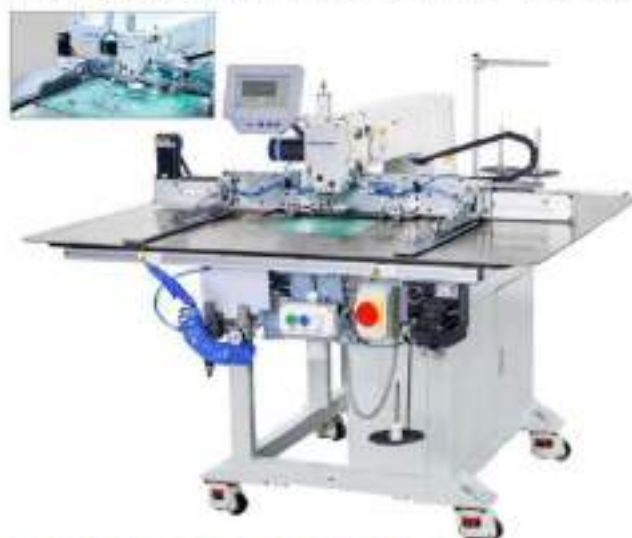
UN8100A-6041H-D (600x410mm) for footwear and leather sewing
