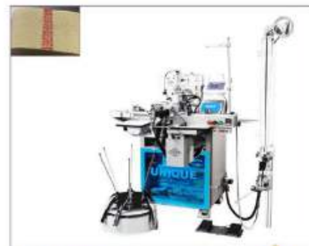
UN-A200P-U Full automatic elastic joining machine with auto feeding, ultrasonic cutting and logo positioning. Auto over-knotting and length measuring Max. elastic width: 7cm Min. elastic circumference: 20cm
