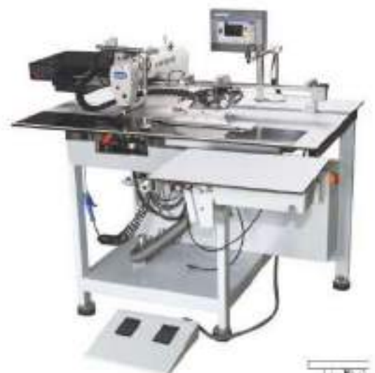
UN-EM2050 Automatic trousers left fly sewing machine Topstitching the left fly piece on men's trousers.
