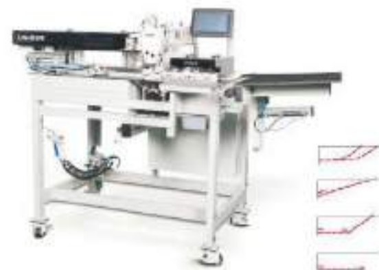
UN-9407 Automatic trousers dart and waistband pleat sewing machine
