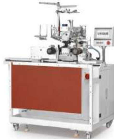
GK-346-2 Automatic coverstitch machine for coverstitch elastic waistband
