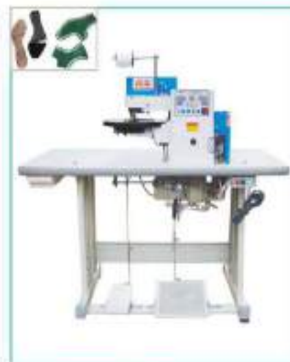
UN-CM998 Computerized hot-cement edge folding machine
