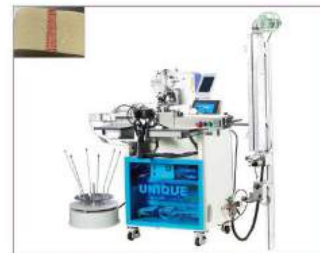
UN-A200B-X Full automatic elastic joining machine with auto feeding, cutting and logo positioning. Auto over-knotting and length measuring Max. elastic width: 5cm Min. elastic circumference: 20cm
