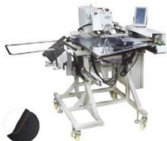
UN2210G-MJ Electronic pattern sewing machine for jean's J stitch 22*10cm UN2210G-MJ 1 needle UN2210G-MJ-2N 2 needles 2 color
