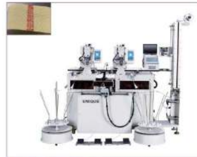
UN-A300B-2-U Full automatic double-station elastic joining machine with auto feeding, ultrasonic cutting and logo positioning. Auto over-knotting and length measuring Max. elastic width: 5cm Min. elastic circumference: 20cm Optional: industrial camera for color sensor
